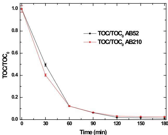
Fig. 6. Behavior of the TOC/TOC<sub>0</sub> during the plasma treatment.
