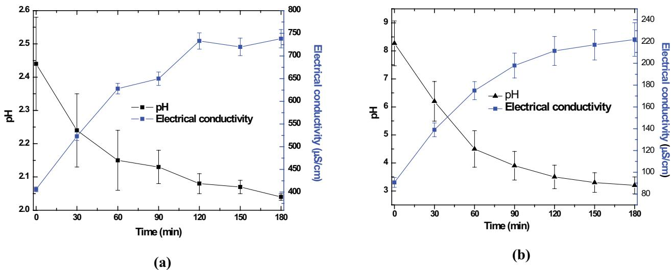
Fig. 3. Behavior of pH and electrical conductivity in the process of degradation of the 2 dyes (a) AB52 and (b) AB210, by plasma.
