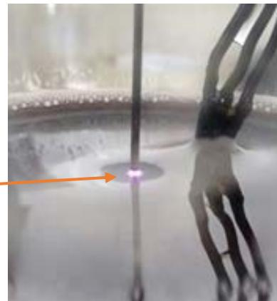
Fig. 1. Reactor for the treatment with atmospheric pressure plasma.
