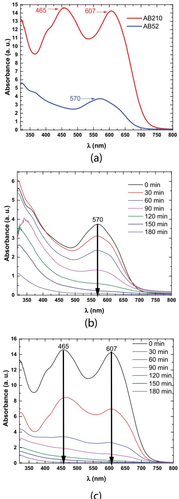
Fig. 2. (a) Initial absorption spectrum of the dyes, (b) degradation process of AB210 and (c) degradation process of AB52.
