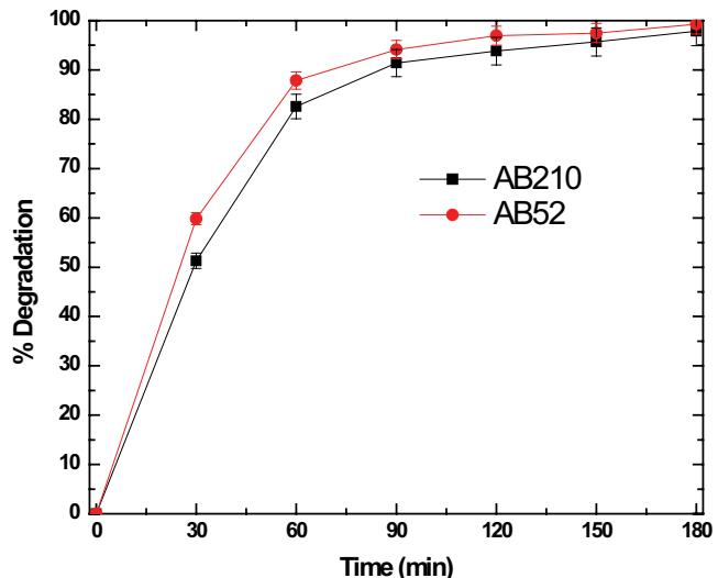
Fig. 4. Percentage of degradation of the dyes as a function of the time of treatment with plasma.
