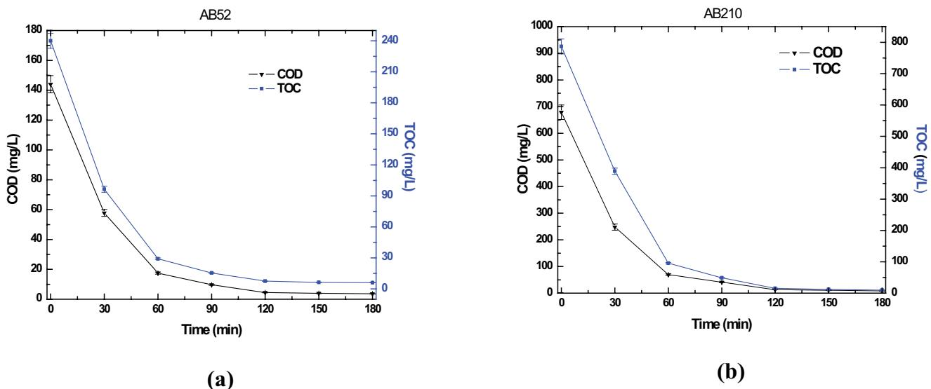
Fig. 5. Behavior of the chemical oxygen demand and total organic carbon during the treatment, (a) AB52 and (b) AB210.
