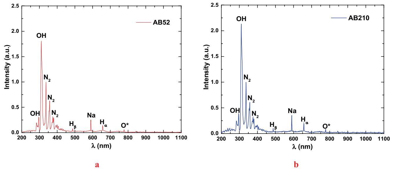
Fig. 8. Optical emission spectrum of plasma by (a) AB52 and (b) AB210 treatment.
